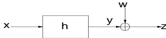
Figure 1.2: The discrete-time channel model.
